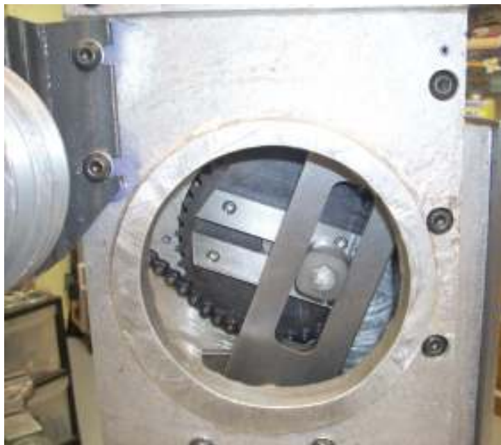
The crank yoke is in the maximum forward position. You can see the scotch yoke through the hole along with the bull wheel.
