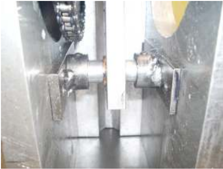
All four screws have been installed and the crank yoke is securely in position.
