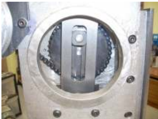
This is a poor man's movie. The yoke is vertical with the crank pin at the top of its stroke.
