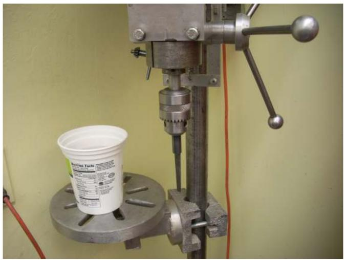
I asked a lot of people for advice on how to make this D reamer. One expert said to not hold the torch on the part too long or it would warp. Another suggested mounting it in a drill press and run the part at 200 RPM while heating and quenching it. Both ideas made a lot of sense to me so I did both. The only problem was that I really didn't know how long to hold the torch on the part. Oh well, that never stopped me before.
