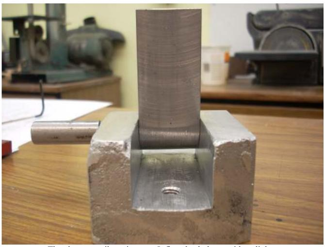
The clapper easily swings up. It flops back down with a slight push. All that is left here is to trim off the excess pivot pin.
