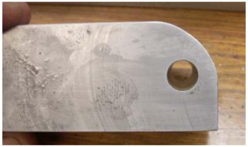
The clapper block came out nice and smooth too. The gunge you see came off of my fingers. The sides of this clapper were lapped nice and smooth.
