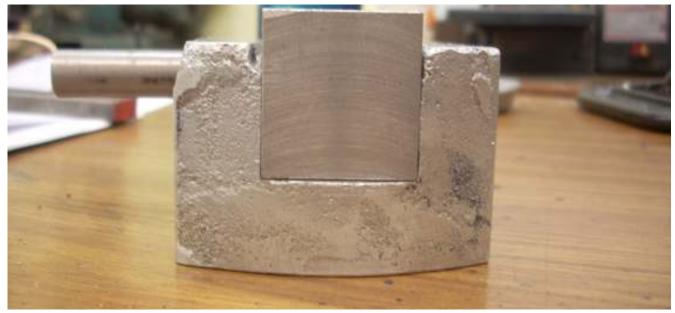
The pin is a snug fit in the clapper box and a sliding fit in the clapper. Dumb luck! Since the pin was cut with the clapper clamped to the clapper box, there is a close fit between the two as can be seen above.
