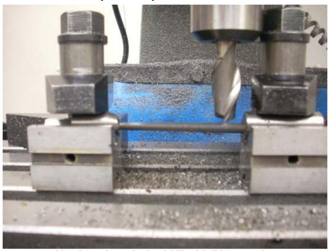
Although I used water hardened drill rod, it didn't cut much different than my CRS. After turning the taper, I moved the part to my mill and put it up on precision V blocks. I knew the diameter was 0.500" so milled down 0.250" to get my D cross section. Because there was uncut stock at each end, it was easy to fixture.
