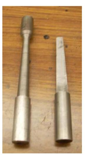
The D reamer is ready to go. To its left is the CRS pin waiting to have the end cut off.
