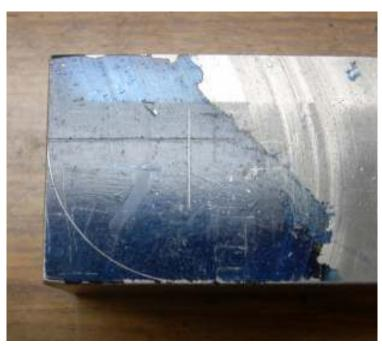
I just realized that I forgot to mention how I cut the radius on the clapper. This radius provides relief so the clapper can swing out without hitting the back of the box.
