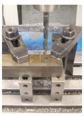
The next test of the reamer was in some 12L14 leaded steel. This is the same material used to make my clapper.
