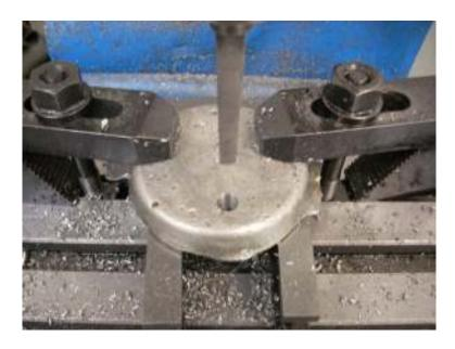
Starting with a "T" letter drill with a diameter of 0.358", I calculated a depth of -0.148". I line up the lip of the drill at the surface of the hole, set my DRO's Z axis to 0, and feed down until I read -0.148". It is only difficult because I chose to use every available drill which turned out to be 22 drills. It is easy
