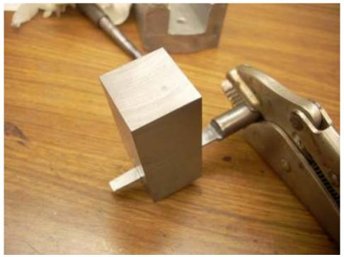
It was then a simple matter to use the reamer to gently remove a tiny amount from just the clapper's hole.
