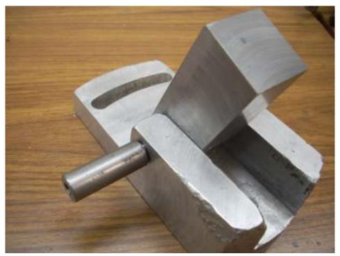
Duh, turned out the minimum diameter of the pin was larger than the minimum diameter of the hole! A quick pass with a 1/4" drill and the pin went in all the way.
