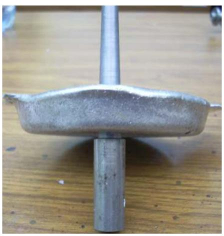
The reamer worked great in the 1/2" thick cast aluminum ingot. My tapered pin was a nice snug fit.
