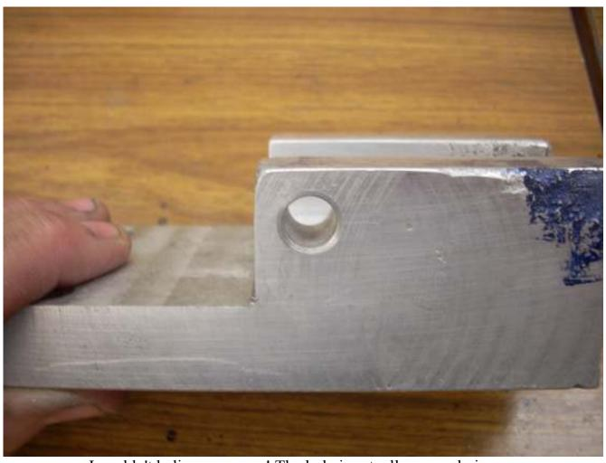
I couldn't believe my eyes! The hole is actually reamed nice and smooth. The chamfer was added after reaming.
