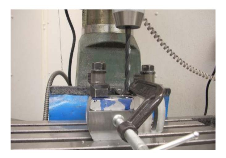
The clapper box and clapper are secured to the table. The C-clamp is holding the clapper tight to the back of the box. This will insure that the clapper is snug against the back of the box during the cutting stroke. Any play would translate into a poor finish.
