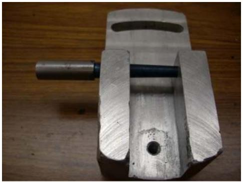
As you can see in this picture, the pin is not seated all the way in. I didn't notice this until after publishing version 1 of this article. I was doing the final fit of my tapered pin yesterday and noticed that it would not go in the last 1/8". At a taper of 0.027" per inch, this means there is a gap of 0.027/8 = 0.003" which is enough play to probably cause chatter.
