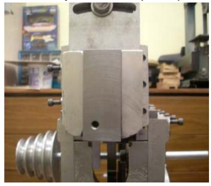
His design places the cutter on the center line of the pivot pin in order to minimize chatter.
