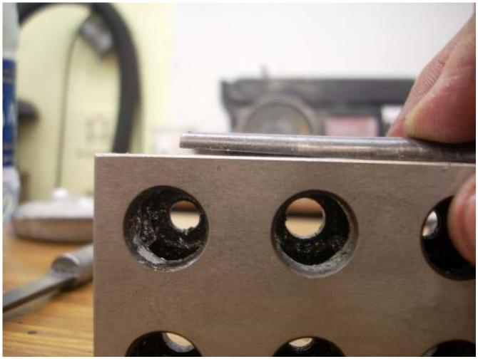
Then I noticed that my reamer was very badly warped, probably during heat treating<sup>2</sup>. No wonder it worked fine in 1/2" thick stock but poorly in the thicker 12L14. Oh well. Time to try again after taking a break. I needed some time to readjust my attitude so I didn't start to feel frustrated.
