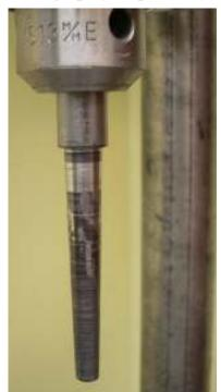
Before I did any damage, I blued the pin and wrung it in the hole.
