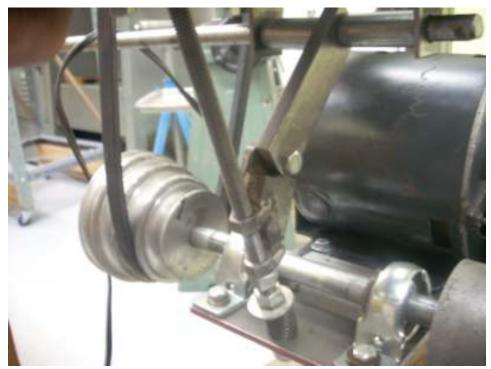
Here you see the belt tensioner in the released state. I can roll the belt along the cone without too much trouble but the task is made easier if I pull the threaded rod forward a bit as shown here.
