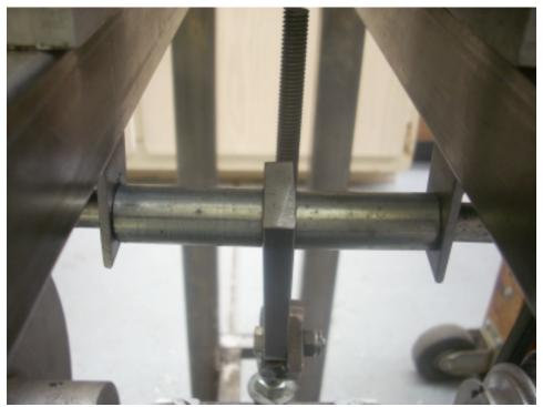
Looking down from the back of the shaper you can see some of the belt tensioner better. The ½" rod is supported by 1" pieces of angle stock that share bolts with the mounting flanges of the column. I hope to bolt an oil pan down here. It would go between the bottom of the top stand rails and these pieces of angle stock.
