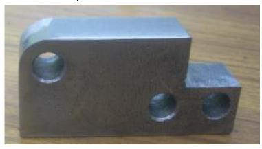
This turned out to be enough metal removed so I moved over to the belt sander for a final rounding.
