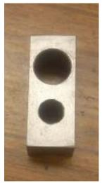
The large hole passes the ram clamp while the smaller hole is for a screw that fastens it to the bottom of the ram (see page 67 of Gingery's book). By just removing the screw and rotating the block, I was able to gain over ½".
