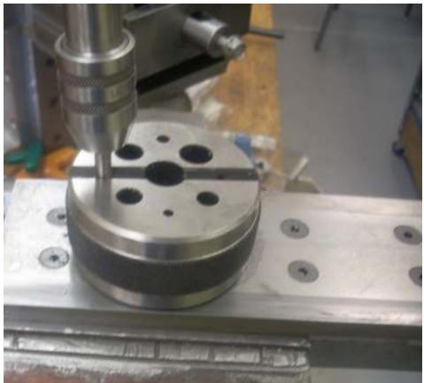
Here I am using a bench block to tap the new hole in the ram ways for the clamp guide screw.
