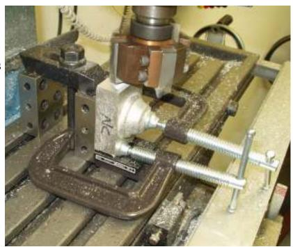
The last machining step was to put the cap down on the table and clean up the top in preparation for the pivot screw and the 4 bolts.
