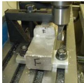
The vertical surface is now done. I could switch to my shell mill for the horizontal surface but it is so small, I will just do it with the end mill.
