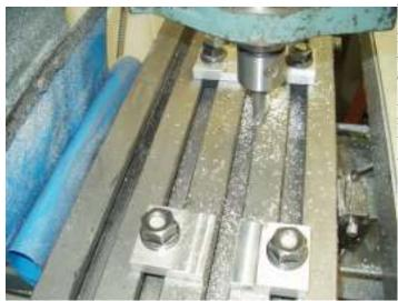
best support the ram casting. The end mill is then used to take a light cut on the horizontal and vertical surfaces. This insures that the casting will be parallel to the table and parallel to the X axis. It is essential that all surfaces are free of swarf.
