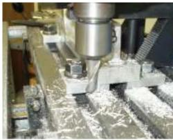
The ram cap pocket is done next. I would prefer to not side mill the vertical part of the pocket but don't see any choice. By making repeated passes without advancing the table, I will be able to remove essentially all cutter flexure.
