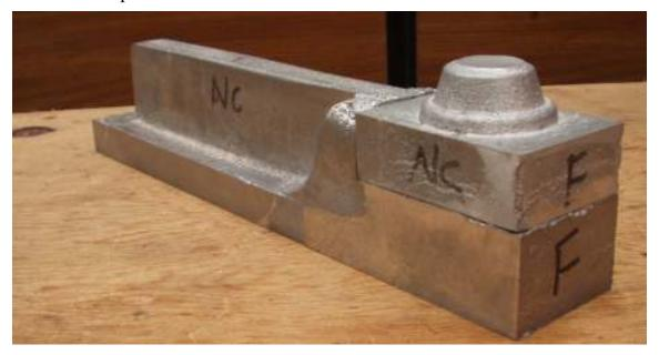
The front will be squared up on the lathe and the sides are not critical. Cap and its pocket are a very nice fit. I see no light between the surfaces.
