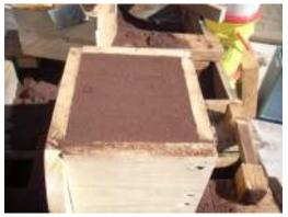
The bottom of the drag has been struck off.
