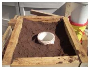
Before I started to ram up the cope, I decided to go with a larger sprue which would also provide extra melt if necessary. I just dropped a piece of PVC over the wooden sprue.
