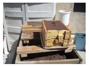
After the pour, I waited about 1 hour before opening the pulley flask. During this time I rammed up the next part. In 7 hours I make a total of 6 pours. The flask you see here contains the rotating head (page 74 in Gingery's book 3). This is my oldest and most worn out flask. During the pour I had melt leak out the sides. What made it a bit painful is that this pattern has a cast in steel core. I ended up just throwing it back into the crucible.
