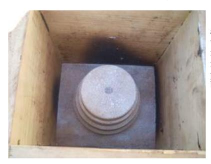
I built a flask that is 8" square and about 14" tall. It permits me to cast the pulley with vertical room to spare. Here you see the molding board with the pulley pattern on top. All surfaces have been dusted.
