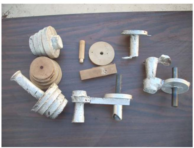
Here is my fun for the day. I cast two pulley blanks, the rotating head in the center (page 74), the protractor on the right (page 77), and feed crank in the upper right (page 68). I sure got a lot of mileage out of just a few patterns.
