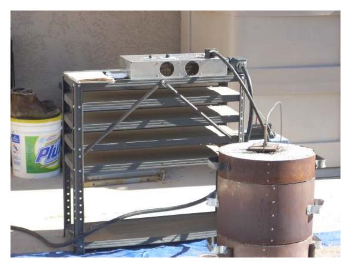
My furnace is a Hartman electric. My controller is the over sized box with the two big cables connected to it. I also have a thermocouple which feeds through the lid of the furnace and into my crucible. I have been running with it in the melt at all times and see no problems so far. It is nice to constantly monitor the melt and see where I am in the process. I was able to see small but sudden drops in temperature as chunks of ingot dropped into the melt. The phase change is very distinctive.
