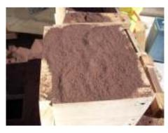
I then sprinkled it with loose Petrobond. I use a flour sifter both for the Petrobond that is in contact with the pattern and for sprinkling on the bottom of the drag. You can see my main tool for pounding the Petrobond on the right side of the picture.
