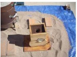
The flask is in position. Note that the cavity is rather large so I will be pouring at the minimum temperature of 632° C. Even at that, there will be a lot of heat in this small area.
