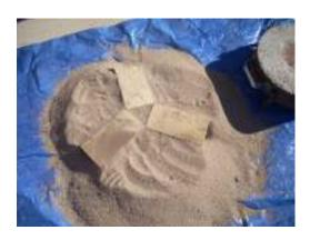
After placing firebricks down to support the furnace, I pour on a layer of sand. Any aluminum that leaks out of the furnace will hit this sand first. Note that the small triangle formed by the ends of the bricks is full of sand. Not a good area to miss. Additional bricks are placed for the crucible and lid.
