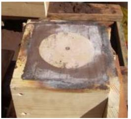
Once the drag has been turned over and the molding board removed, you can see the top face of the pulley pattern. There is not a lot of clearance between the pattern and the flask. Note the minor burn marks on the wood. The flask has plenty of depth but would have been better if made a bit wider.
