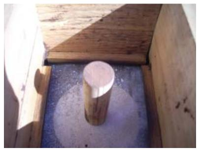
With the cope in place, I set the sprue. When I cast this pulley the last time, it did not have a riser and there was no shrink problems.
