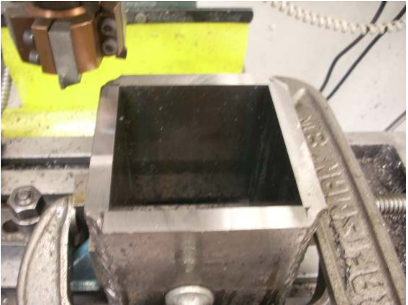
First end done and ready to turn the box over to true up the side that will take the end plate.
