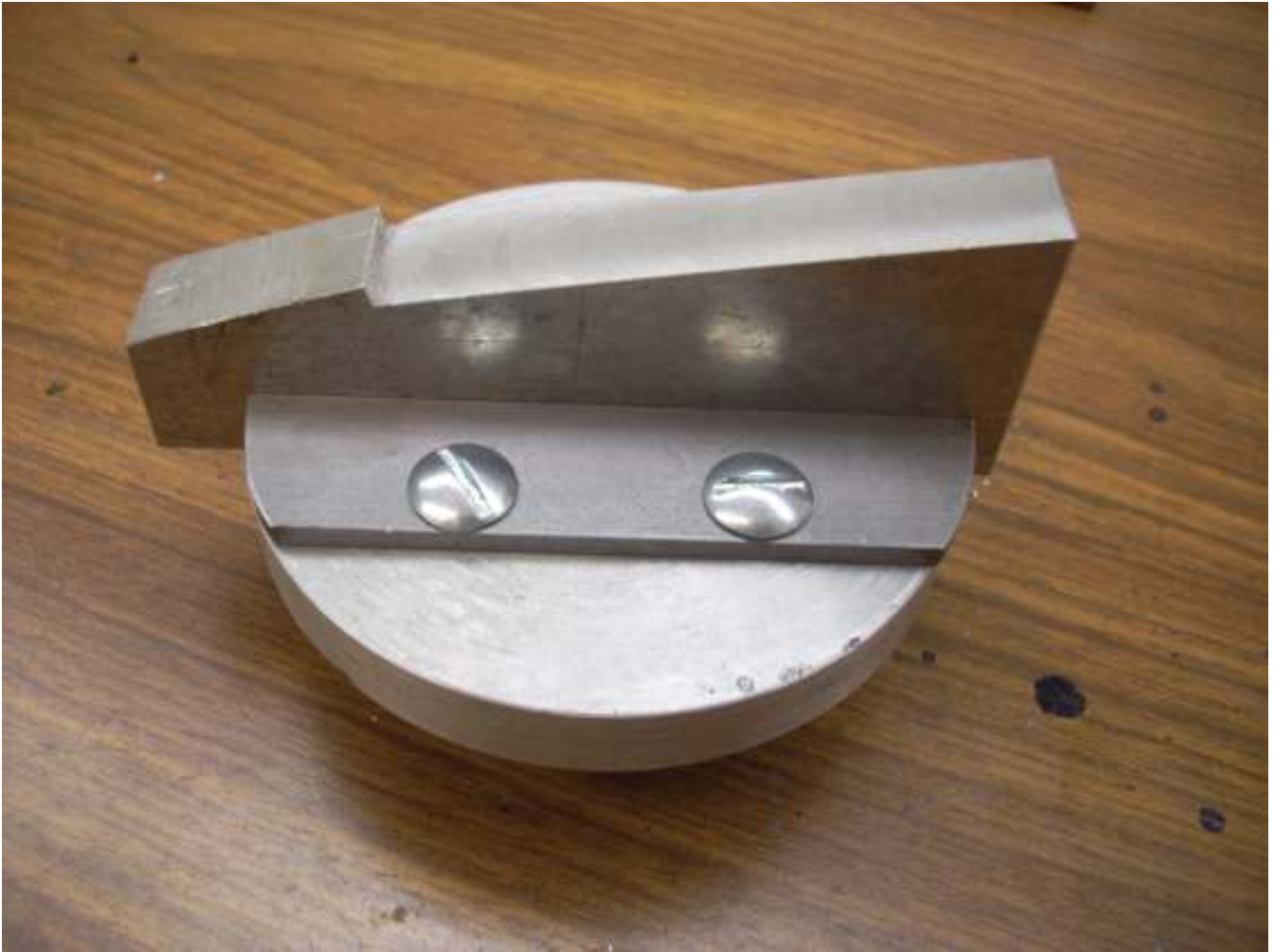
With the 0.500" spacer back into the slot, I do my final fitting of the first plate.
