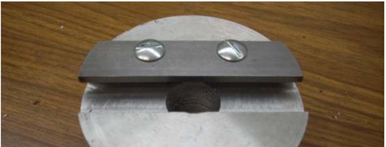
With the 0.500" spacer back into the slot, I do my final fitting of the first plate.
