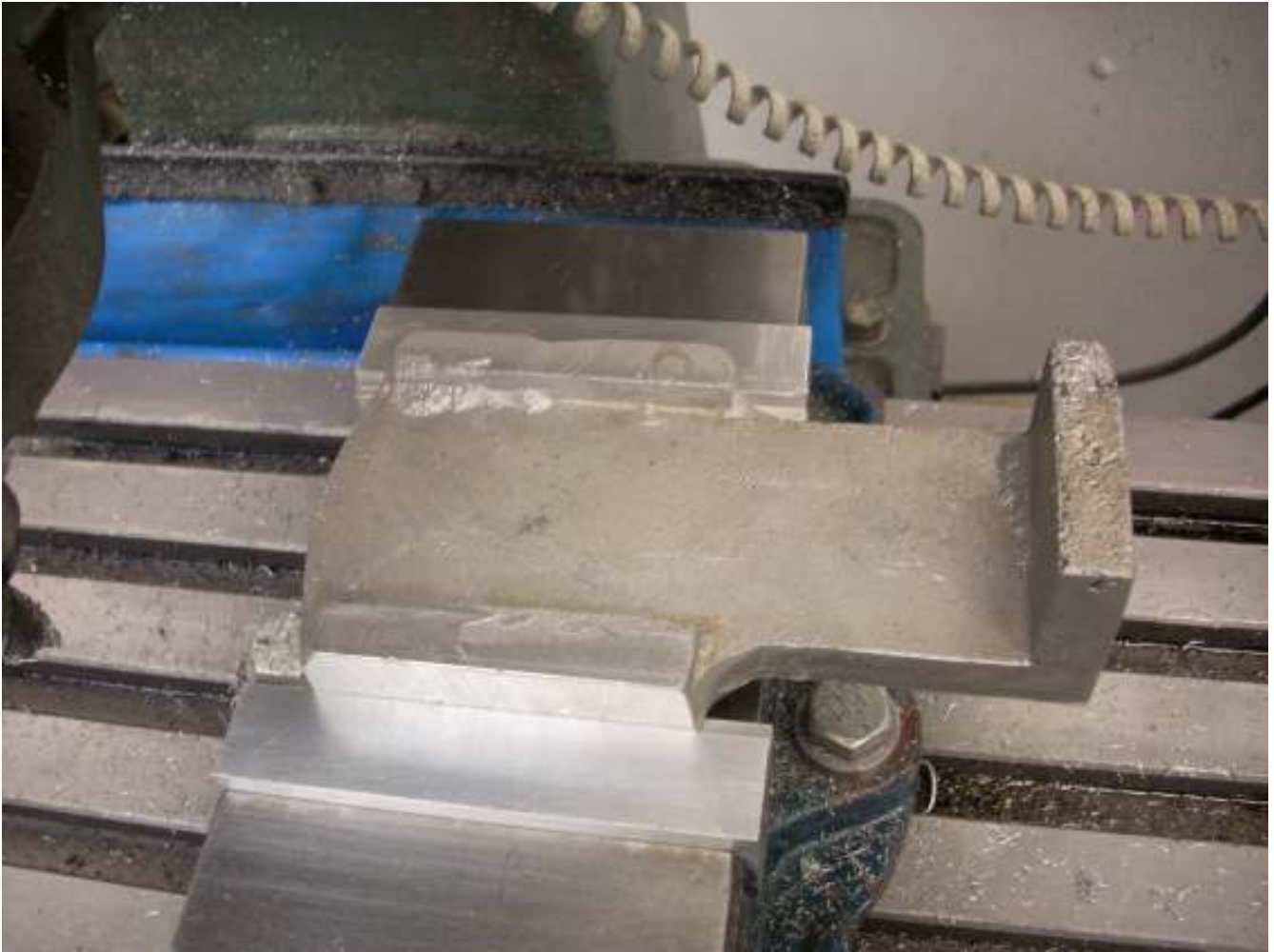
The casting is now securely held by my soft jaws on Reference 2 and 2 prime. Reference 1 is parallel to the mill table.
