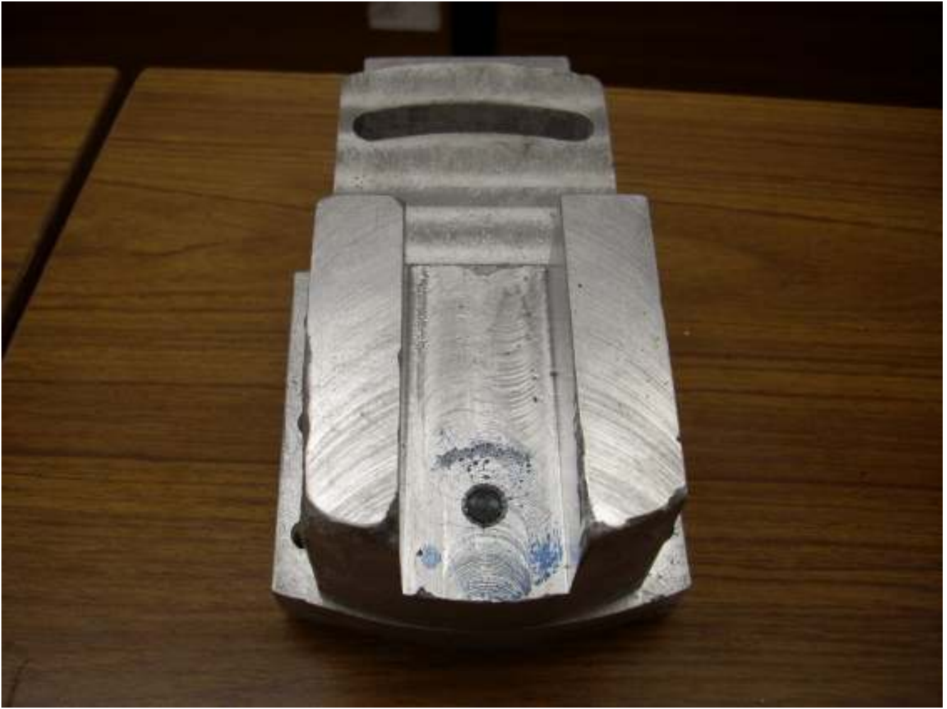
The part was put back in my vise and the surface milled.
