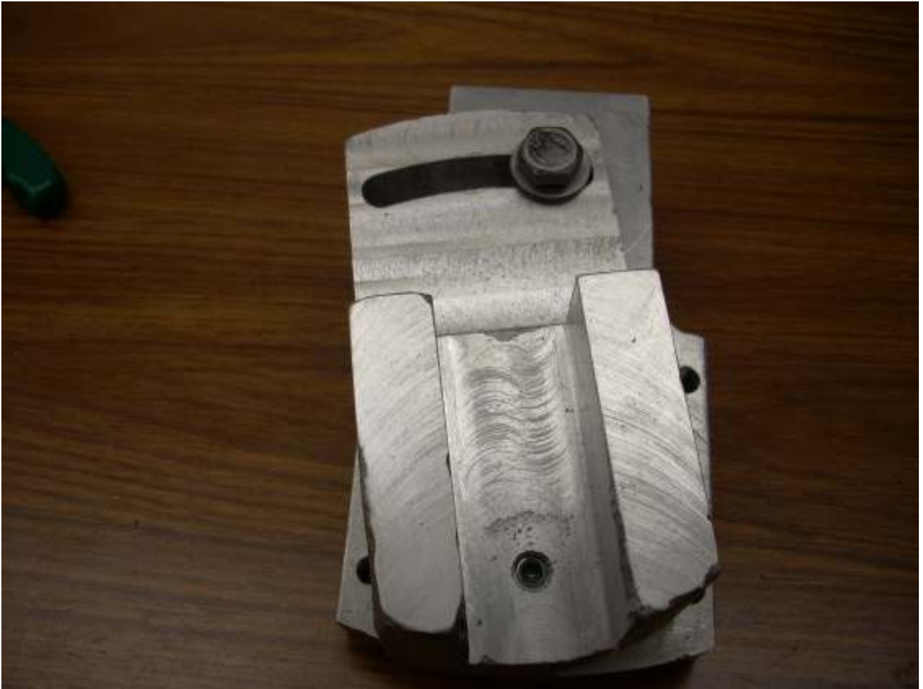
With the screw installed, you can see that I am able to swing the clapper box all the way to the left.
