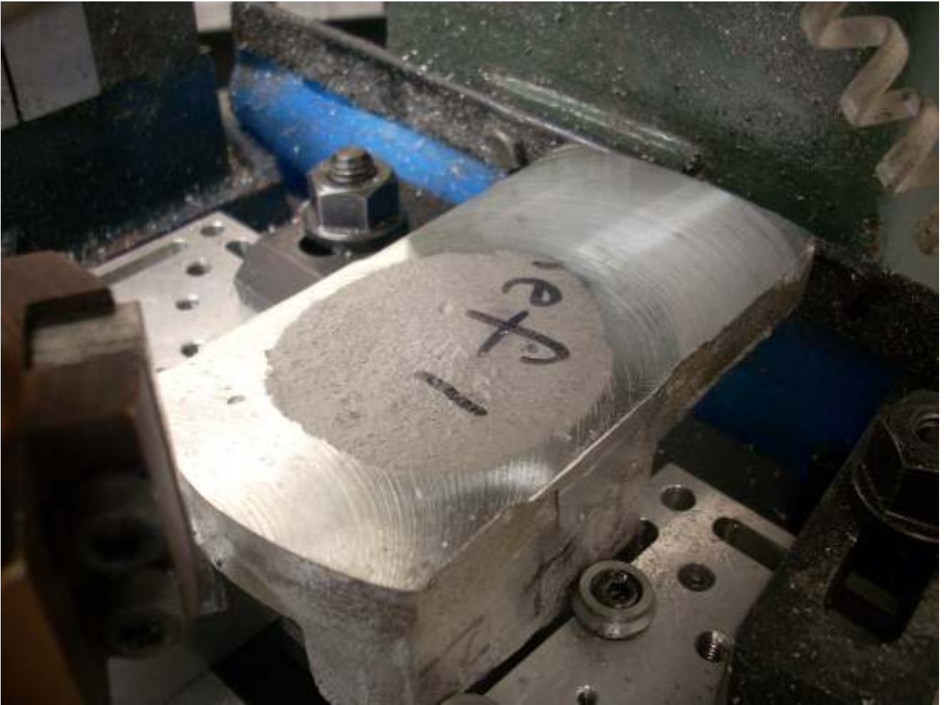
After the first pass you can clearly see a bit of shrinkage. Fortunately I have plenty of metal here so can afford to cut deeper.
