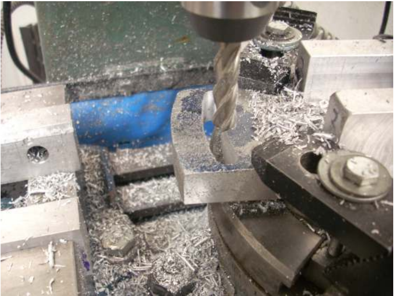
The slot is then side milled. I moved the rotary table from -14^{\circ} to +14^{\circ} and get a nice looking arc.
