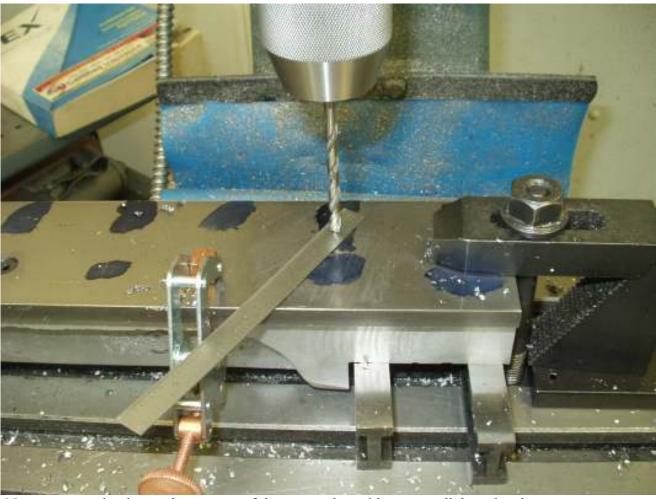
Now you can clearly see the support of the cap pocket with two parallels and a clamp.
