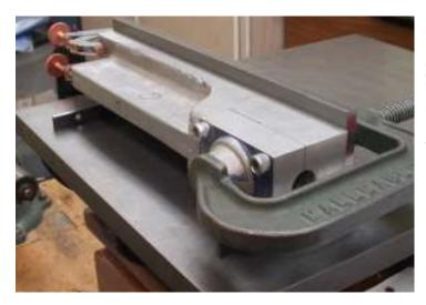
The CRS plate was inspected for burrs and cleaned up as needed with a file. I placed it down on the surface plate to verify it was dead flat. It was then placed on edge on the surface plate and clamped. The front edge of the plate is about 1/16" back from the front of the casting. This offset permits the down feed assembly to contact only the casting.
