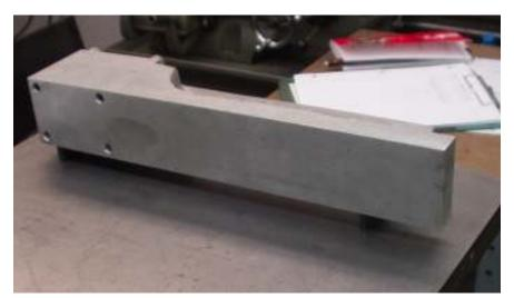
Today I started to attach the CRS plate to the bottom of the ram casting. Gingery calls for 1/4" thick plate but I have chosen 3/8" for added rigidity.
