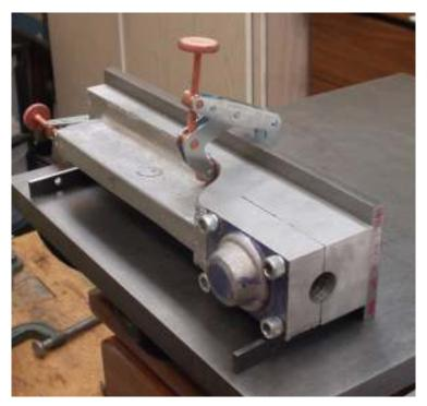
Back to the surface plate where I moved one of the smaller clamps. I was still not happy because I have no simple reference surface facing the mill table.
