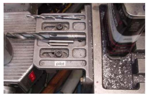
A justified fear for me is that I confuse the different drills. I have learned the hard way that it is best to call out "clearance" and "pilot" in my procedures. Then I place the proper drill in the little marked pockets. I have the pilot drill chucked so you see the reminder tag. There is just a limit to what I can focus on at the same time. Anything that moves me towards fool proof is a help.
