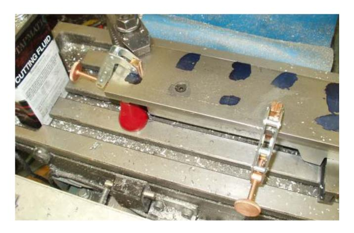
The casting can now easily be set up on the mill table. On the right end you see one of two parallels that support the cap pocket's reference surface. I clamped this end down first and then placed jacks on the other end of the casting so they are snug. The plate with casting was set parallel to the X-axis by mounting a spud into the drill chuck and sighting its point along the edge. I am drilling bolt holes here so being with 10 thou is acceptable.
