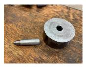
Unisawyer made up pair of "presser plates" (timestamp 9:23) with the back turned down to 3/8". I had a puck of CRS in my junk drawer. I drilled and reamed it 3/8" and then pushed a pin into the hole. It won't be as strong as a turned down spigot but will be fine as long as I don't push too hard on the unsupported part of the face.
