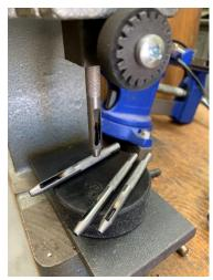
The next attachment inspired by Unisawyer was a set of punches. I had these hand punches and found that they fit into the bore. I'm using a hockey puck to support the stock as I punch through. If this is too soft a surface, I have some expanded PVC, a piece of hardwood, and some brass. One of them should work.
