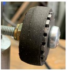
This picture also shows my locking screw. Unisawyer suggested using a set screw that is below the surface of the ram. This is a metric thread and I didn't have a matching set screw<sup>2</sup>. I could have drilled out the threaded hole and cut SAE threads. But instead, I made a knob.
