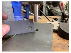
The small hole was punched by the smallest punch shown above. The large hole was from the rod and plate arrangement.
