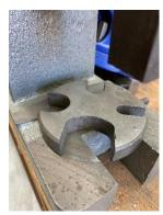
The one attachment that came with the press was this disk. I never needed the cutouts and when I used a patch of the solid area, the disk would rock. It didn't give me a lot of confidence.
