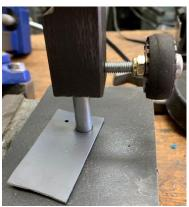
With some scrap waterproof membrane down on the plate, it was easy to drive the rod through.
