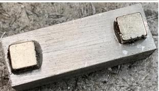
I thought up many hard ways to correct for letter rotation relative to the shank before arriving at this solution. You are looking at the end of a ½ X ½ X 1 inch block of aluminum. A **21/64 inch** hole is drilled through, a little off center.
