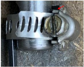
The allen wrench fits through the hole (red arrow) and the hose clamp secures it to the rod.
