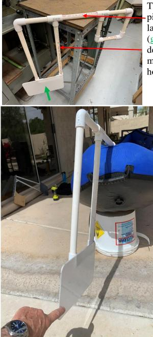
The weakest part of the frame is the horizontal pipe running between the small square and the large rectangle. A side force applied to the skeg (green arrow) acts through those long pipes that define the large rectangle so there is a large mechanical advantage here that will twist that horizontal pipe. So how bad is it?
