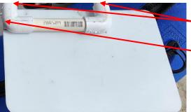
8. Place the assembly on the plate, flat side down. The top of each coupler is aligned with the top edge of the plate.
