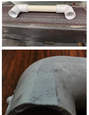
7. If you have a belt sander, gently place the assembly down on the moving belt and abrade off flats on the flanks of the couplers. The goal is to have two "L" shaped flats about ¼ inch wide.
