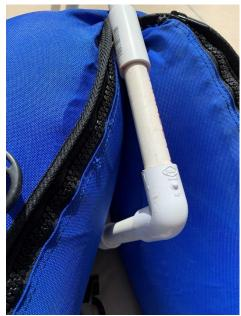
After fully inflating the kayak, slide the square part of the frame between the gunnels at the stern. Run a tether from this square part to a D ring on the gunnel. We don't want to lose the skeg *when* the kayak capsizes.
