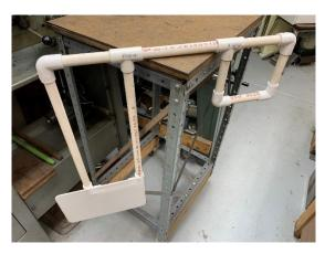
11. Complete the assembly process being careful to keep all pipes and couplers on the same plane.12.Give the PVC cement about 1 hour to fully set before stressing the joints.13.Optionally, spray paint the frame and skeg.
