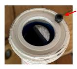
The solution was to add a pin to one side of each union and drill a matching hole on the other side. I drilled and tapped the first hole 6-32 and installed a Socket Head Cap Screw. The other hole was drilled large enough to easily accept the screw's head.
