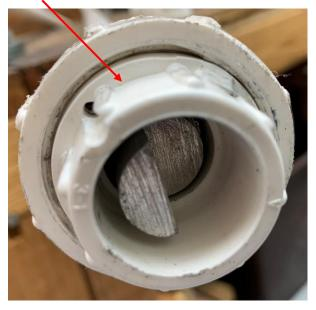
Then I drilled into the face with my tap drill going through my previously drilled hole.
