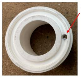
I took a spare PVC union and drilled a tap hole in the desired location.
