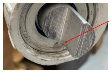
Then I took a drill that was a loose fit to the screw head and mounted it in my pin vise. I used it to open out the tap hole on the opposite side of each union. I had far better control of the drill with the pin vise than using my hand drill.
