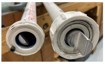
Recently I built a tool for my neighbor for use at a wastewater treatment plant. When assembled from four pieces, it is 20 feet long. Turn a handle on top, and a chamber closes at the bottom.
