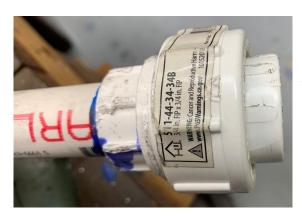
With the drill guide mounted in its threaded collar fitted on the end of the section, I drilled through with my tap drill.
