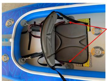
Second, I added a strap, with hooks, at the bottom of the seat. The hooks engage the front D-rings.
