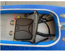
Before I board my kayak, the seatback is vertical, and the front edge of the seat bottom is lined up with the outside of the valve flange (red arrow).
