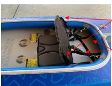
After about 15 minutes of paddling, my butt has walked the seat bottom back a few inches. The front straps are still in tension, so the upper third of the seatback hasn't moved much. But the rear straps are now slack.
