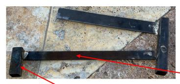
This tool does the trick. The parts are brazed together but they could have been welded. Initially I used Pop Rivets but they were far too weak.
