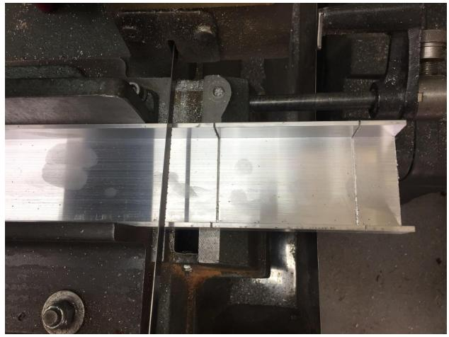
I then slide the channel over by the length of my project and make another cut down to half the thickness. And finally, I slide over another inch. This last cut is all the way through the channel.
