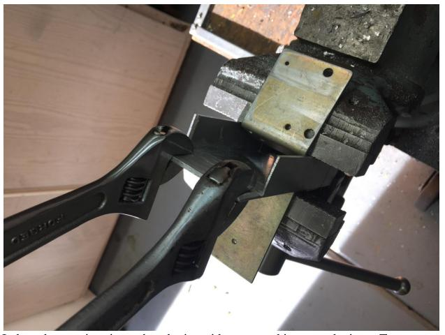
I place the cut piece in my bench vise with some packing over the jaws. Two adjustable wrenches are used to bend the end over. This is repeated on the other end.
