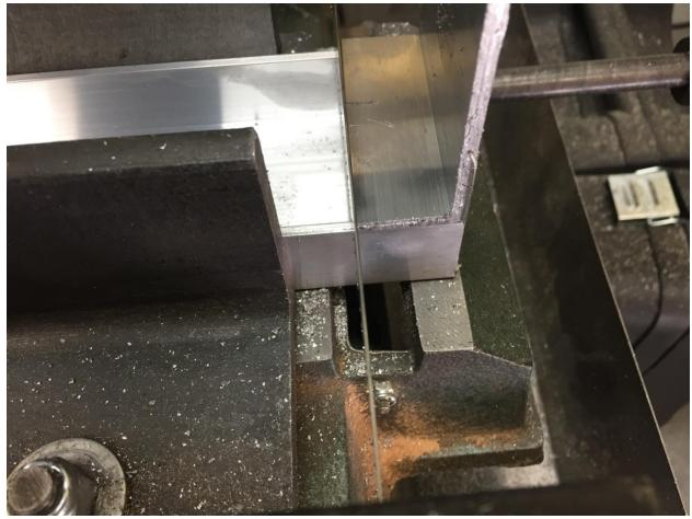
I'm using a piece of scrap channel as my 1-inch ruler. A length of the channel is clamped in my bandsaw with 1 inch beyond the right face of the blade.
