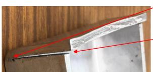
The saw cut has been closed by bending the end.
