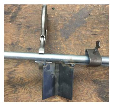
To make the fixture, I started with an 8" length of ½" angle and cut about 2" off the end. Then I clamped the two pieces to a length of EMT conduit. Placing it down on the end of a piece of 2" angle, I adjusted one of the clamps so the two pieces of ½" angle rested flat on the end of the 2" angle.
