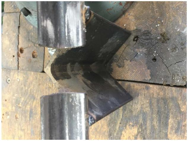
This arrangement gave me a means of aligning two rods of equal diameter while having plenty of room to tack weld. It is best to spray the ½" angle with antispatter before each use.
