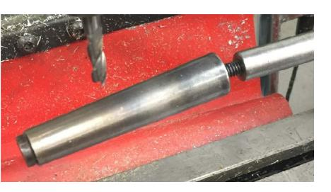
I had a spare tapered shank that fit the taper in the center of my rotary table. I faced the wide end on my lathe. Then I drilled and tapped it  $\frac{1}{4}$  - 20. The taper can be screwed onto the end of the rod and removed at will.
