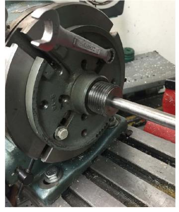
After the threaded section is run into the faceplate, the two mounting screws are tightened.
