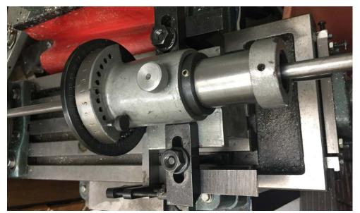
The collet spinner is loosely clamped down on its block.
