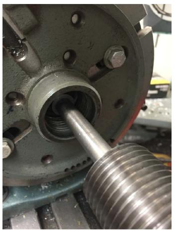
The tapered end slides into the tapered hole in the rotary table.
