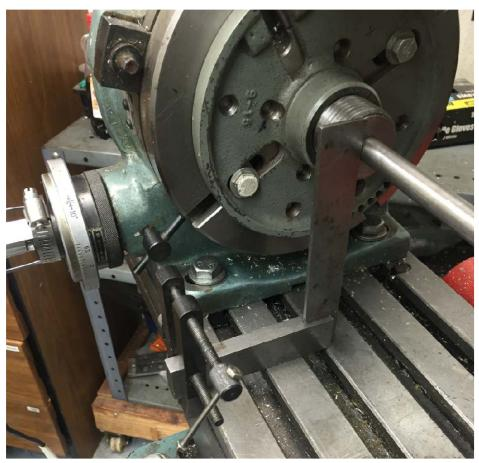
The rotary table has previously been aligned to the front face of the table and locked in place.
