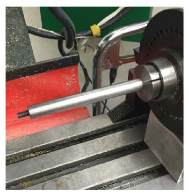
Using my lathe, I faced a piece of ½ inch CRS. Then I drilled and tapped it ¼ - 20 to a depth of about ½ inch. A 1 inch long piece of threaded rod was screwed into the hole. Puzzle piece two.
