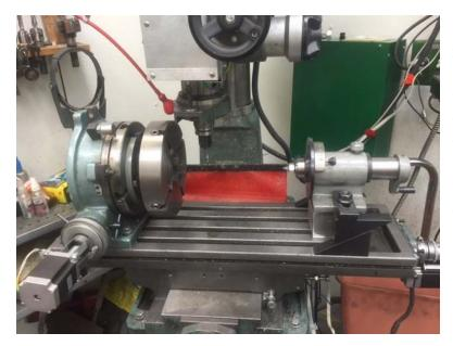
First I converted my 8 inch rotary table into my 4th axis<sup>2</sup>. Then I built the tailstock<sup>3</sup>. The final step was to figure out how to align the tailstock to the rotary table.
