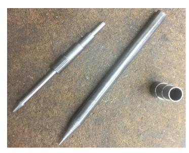
If you reamed the holes, the rods should be a snug sliding fit into the stepped collars. If drilled, they may slide a bit more freely. This will decrease accuracy a little but should be fine.
