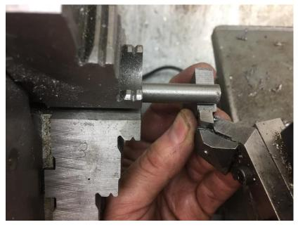
I'm going to be making a lot of 3/8" wide steps that do not have to be very precise. I chose a scrap of 3/8" thick stock to use as a gage. Just eye-ball the cutter's position before each step is cut. *NEVER* do this with the lathe running.
