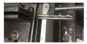
Next, take each rod over to your saw and cut them to the same length as your drill bit of the same diameter. Using a file or sander, smooth the cut end.
