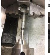
drill has an end like a regular drill but the rest of the body is smooth. It is a good way to cut a cone shaped hole that will later center a drill.
