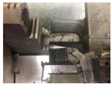
Start by checking that the cutter is right on the center of rotation so the point will be as sharp as possible.
