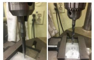
This Drill Location Tool is based on a pointer called a "spud". I'm guessing that the name comes from the spud wrench:
