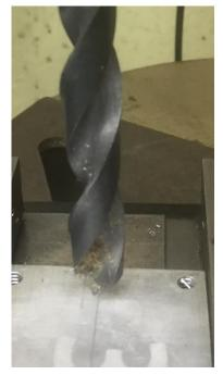
Then drill the hole nicely lined up with the punch mark. This picture shows how difficult it can be to even see the punch mark with the drill over it.
